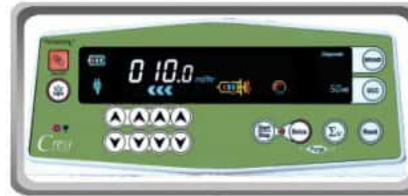
EBTN LCD Display with Capacitive Touch Screen Key pad
